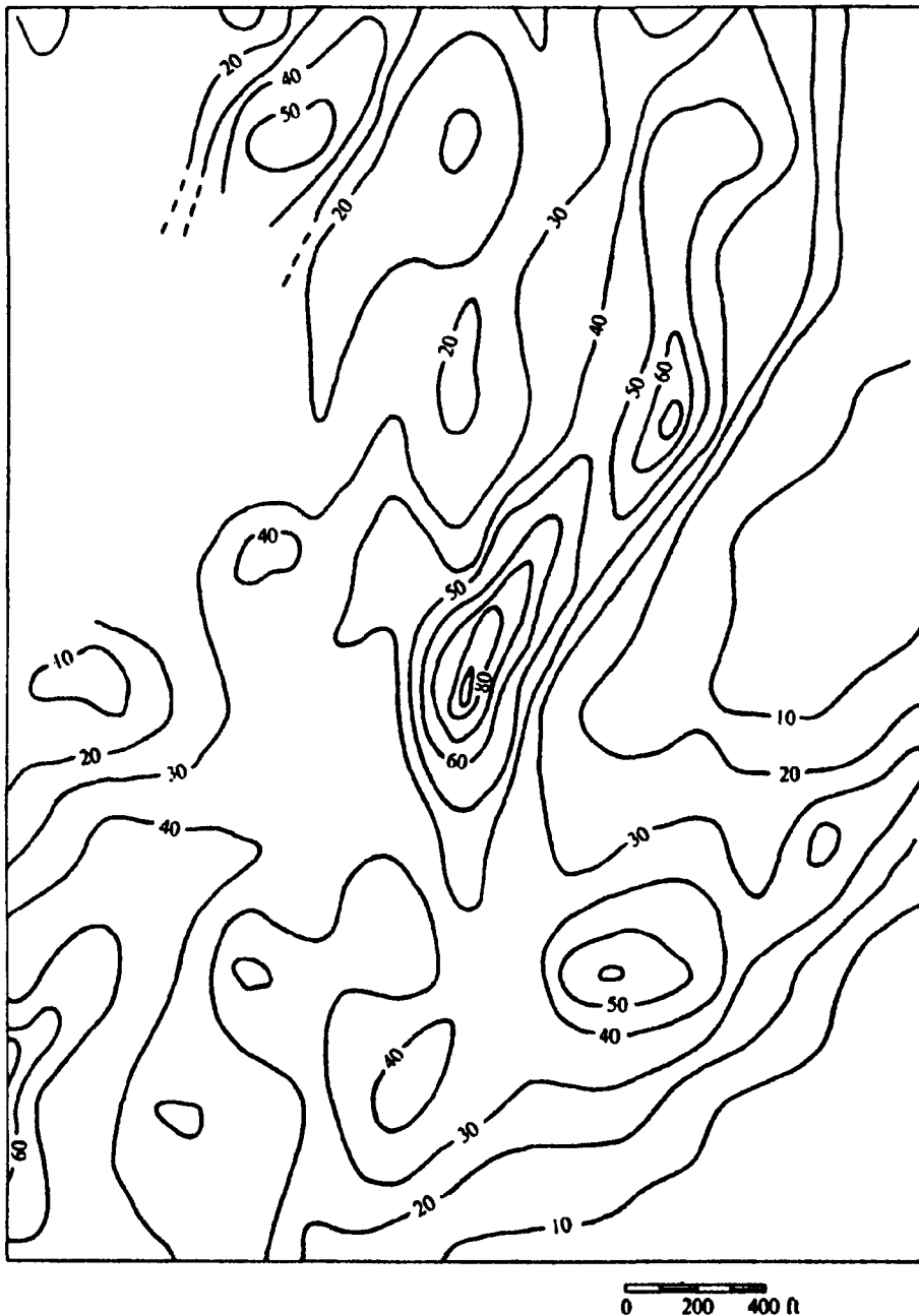
Figure 9.23. Metal-factor contours, double-dipole array: x = 100 ft, n = 1 .
